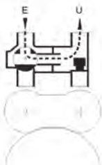
Handmatige bypass - systeem in bypass
