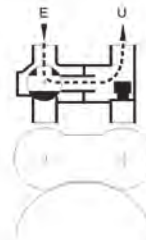
Manueller Bypass - Bypass-Stellung
